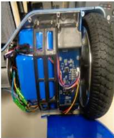
Picture of Lithium Battery Installed within Hoverboard
